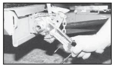
**Step 2.** Ensure that towed vehicle parking brake is fully engaged, then release the tie-down straps. **NOTE:** Tie down straps must be "quick-released" by grasping ratchet pawl and ratchet handle simultaneously and pushing down sharply. This process will permit easy removal of strap from winch. Remove tie-down strap hook from its storage position at the rear of the ramp. Lay the straps on the ground in front of the winches.
